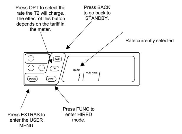
✓ In FOR HIRE mode, the T2 may illuminate the roof sign of your vehicle. This depends, however, on the tariff program in the meter.
