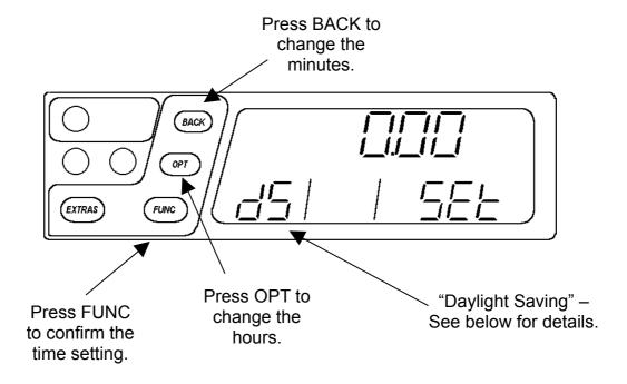
Note: if the letters "dS" are shown in the rate window, the time shown takes account of "daylight saving". This means that the tariff program includes adjustments for Winter and Summer time and that such an adjustment is in force on the date you have entered.
