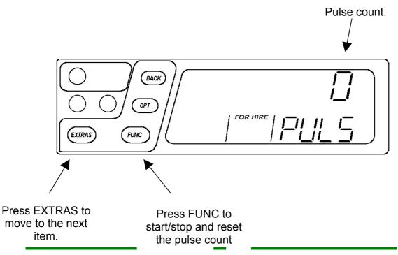
The initial display shows a pulse count of "0" with the text "PULS".
