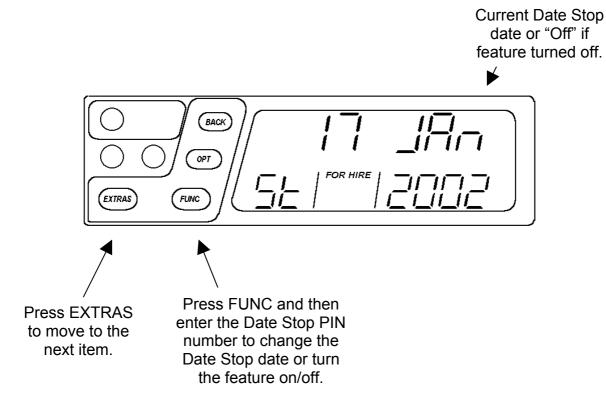
If the Date Stop feature is currently enabled, the date is shown. If it is not currently enabled, the word "OFF" is shown.
