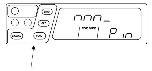
Enter the 6-digit PIN using the buttons for the numbers 1 to 4.
