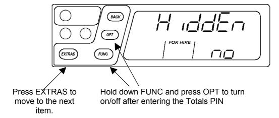
With this option set to "on", the "Permanent" Totals are always hidden from view until the user enters the Totals PIN.
