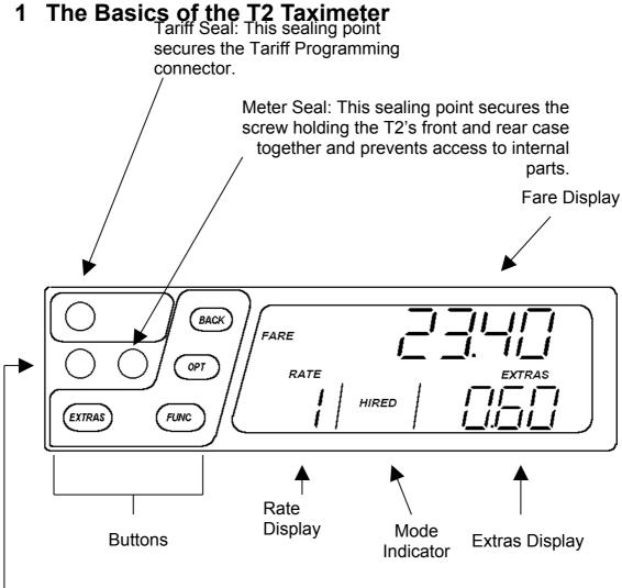
Vehicle Seal: This sealing point secures the screw holding the T2 to its mounting bracket.
