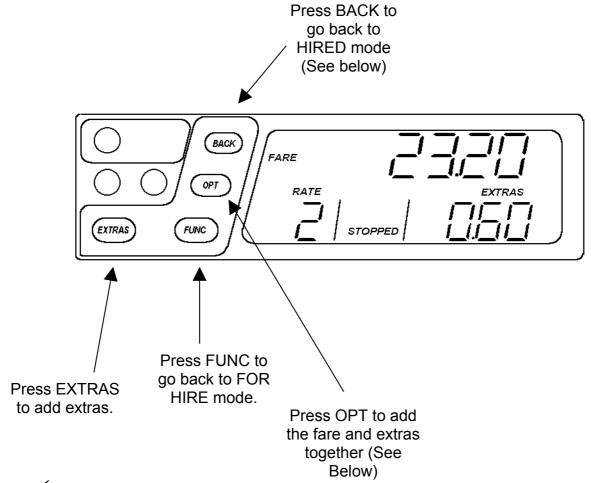
✓ If the T2 is programmed to do so, pressing the OPT button in STOPPED mode will cause the fare and extras to be added together and the legend "TOTAL FARE" to be illuminated. The exact behaviour of this feature has several possible options. If you require any further information, please contact your dealer.
