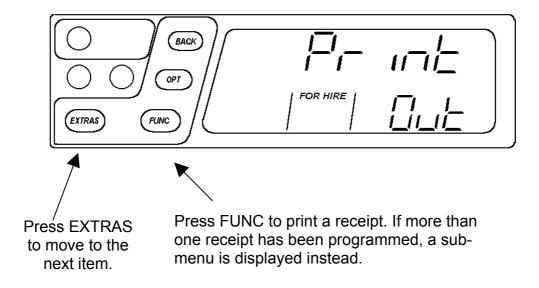
Assuming that a receipt printer is connected to the T2 and switched on, a receipt may be printed:
